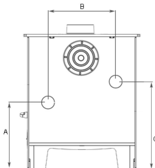
Add In Boiler Tapping Measurements.
