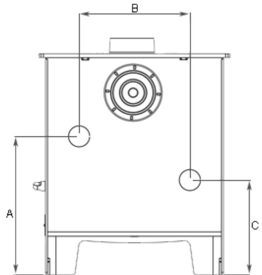
Add In Boiler Tapping Measurements.
