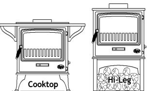
Attach to the underside of the stove using the bolts supplied before fully tightening. Note the 'Installation Clearances' on page 1. When used as a log store, logs must not be placed higher than the central 'bridging' member.
