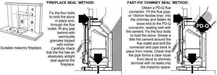
Whichever method is used it is imperative that: (1) The route for gases from the stove to the chimney terminal is completely air-tight; even the tiniest gap or crack can spoil the updraught. Seal all joins with fireproof cement and/or heatproof rope. (2) It is possible to sweep the entire length- access doors may be required. (3) The entire construction is of durable fireproof materials. (4) It is wise to fit a CO alarm.
