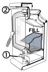
Place two or three firelighters close together, or screwed-up the back of the grate and light them. When they are burning well gently fill the fire with dry fuel, close the door and set the air control slides to the 'high' (right) position. When the fire is burning well, move the controls to the lowest practical setting.
